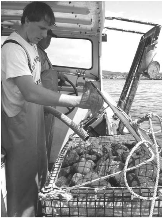
Figure 3. Mimicking nature. Collector on the rail of a lobster boat. This collector was fitted with a fine mesh cover that is being removed after the test to evaluate haul-back losses of postlarval lobsters seeded to the collectors.
