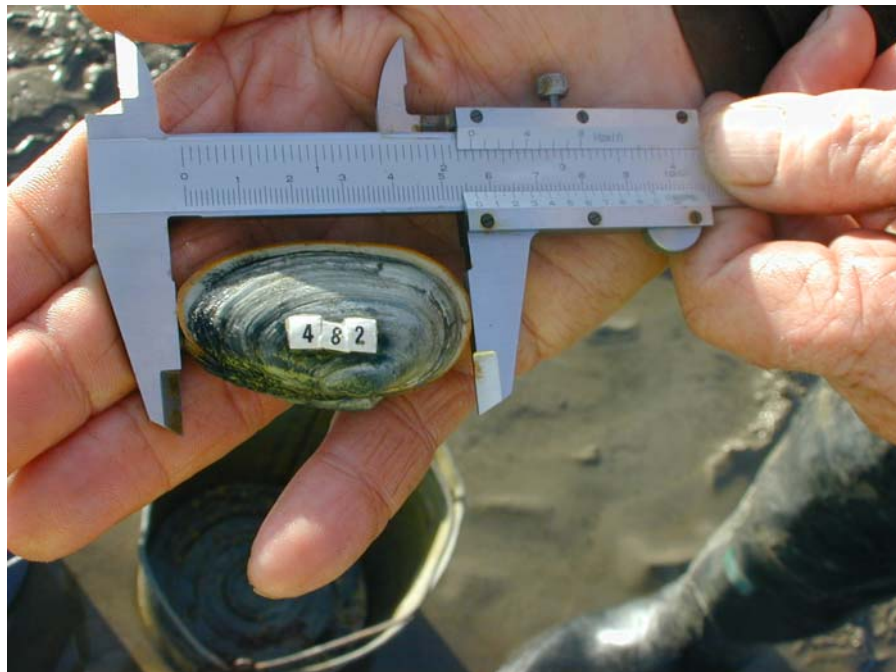
Clams were individually marked, glued with epoxy, then measured with calipers for each sample.
