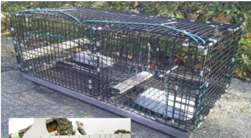
Lobster Recruitment project trap measures 14"x 21"x 40". It has 1 " mesh, no escape vents and a biodegradable panel
